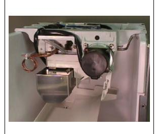
Unlike the initial harvest, the normal harvest is controlled by the thermistor. When the thermistor reaches 59°F, the control board deenergizes the hot gas valve and energizes the condenser fan motor. The actuator motor energizes to raise the plate. When the plate reaches the evaporator, the actuator toggle switch is moved back to the right. The board de-energizes the inlet water valve and the freeze cycle begins again. The average harvest cycle is about 3 minutes.
